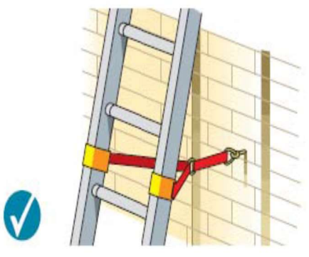
Tying near the base
